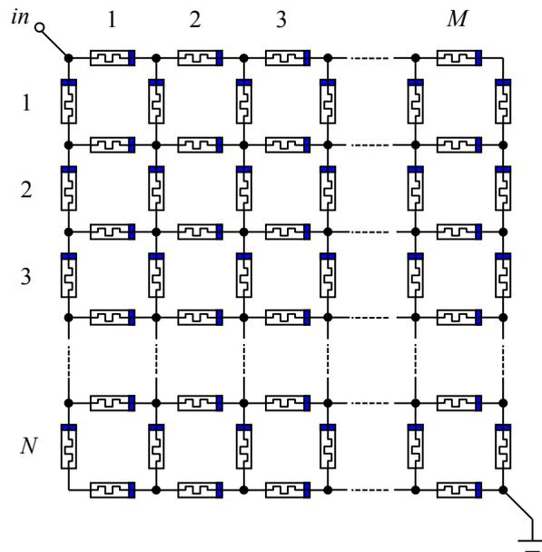
Fig. 3. Benchmark circuit compounded of  $2MN+M+N$  identical memristors.
