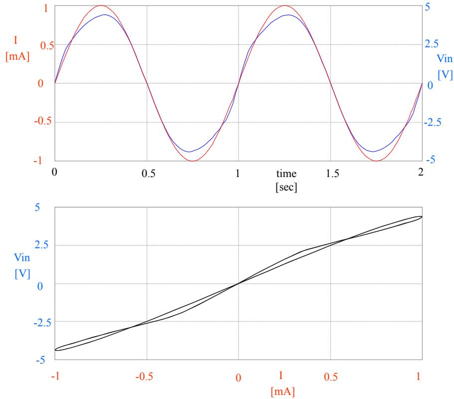
**Fig. 5.** Transient analysis of the circuit from Fig. 3 for  $M=50$ ,  $N=30$ , driven by sinusoidal 1 mA/ 1 Hz current;  $R_{mi} = 1.3 \text{ k}\Omega$ ,  $R_{on} = 100 \Omega$ ,  $R_{off} = 10 \text{ k}\Omega$ ; step ceiling = 0.02 sec.
