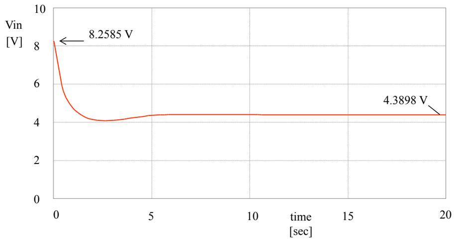
Fig. 4. Results of transient analysis of the circuit from Fig. 3 for  $M=50$ ,  $N=30$ : voltage response to a constant current of  $250 \mu\text{A}$  flowing into the *in* node;  $R_{ini} = 6 \text{ k}\Omega$ ,  $R_{on} = 100\Omega$ ,  $R_{off} = 10\text{k}\Omega$ , step ceiling = 0.2 sec.
