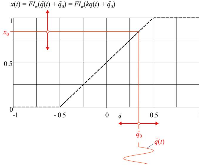
**Fig. 1.** Nonlinear function for transforming the normalized charge  $\bar{q}$  into the normalized physical state variable  $x$  of  $\text{TiO}_2$  memristor with rectangular window.
