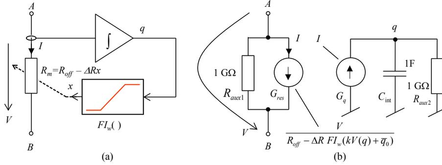
**Fig. 2.** Model of HP memristor. (a) ideological, (b) for SPICE implementation.
