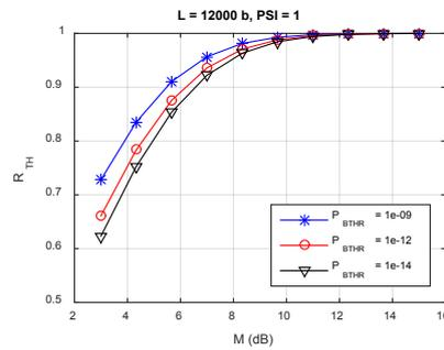
**Fig. 5.** Relative throughput as a function of link margin
