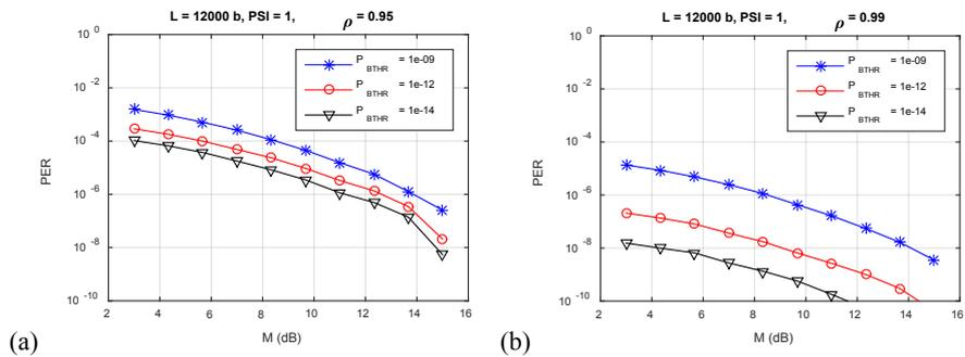
**Fig. 4.** Adaptation unit performance as a function of threshold for (a)  $\rho = 0.95$ ; (b)  $\rho = 0.99$ .
