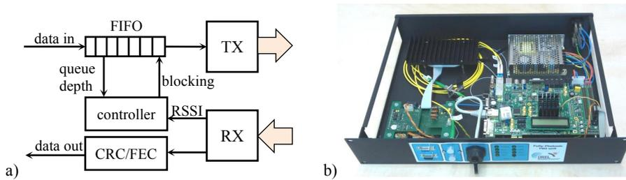
**Fig. 2.** (a) Structure of link adaptation unit; b) Actual implementation based on Virtex-5 FPGA.
