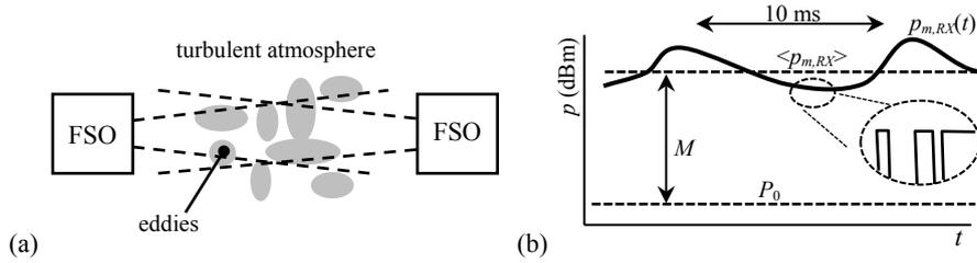
Fig. 1. (a) FSO link configuration; (b) Received power budget model.
